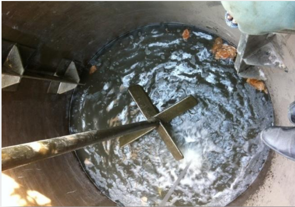
CS/FRP Lined Pitch Blade Turbine Imp.
