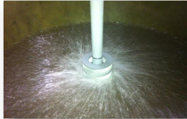
CS/PVC Lined Curve Blade Agitator
